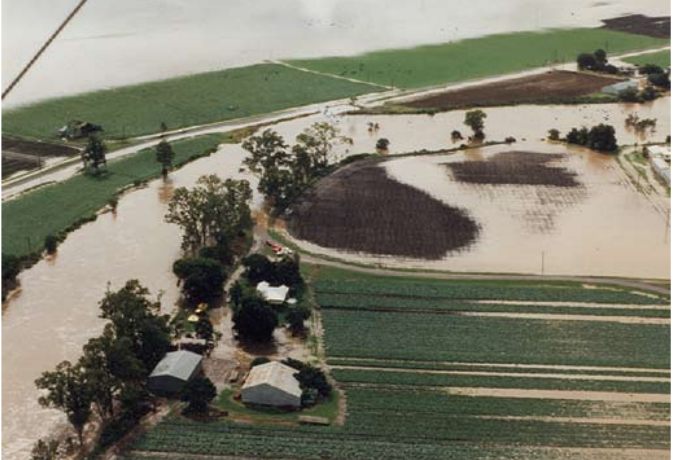
Natural levee: The road at Lockrose rises up over the natural levee bank, protecting its integrity and ensuring that this is not a point of concentrated flow and potential erosion site.
